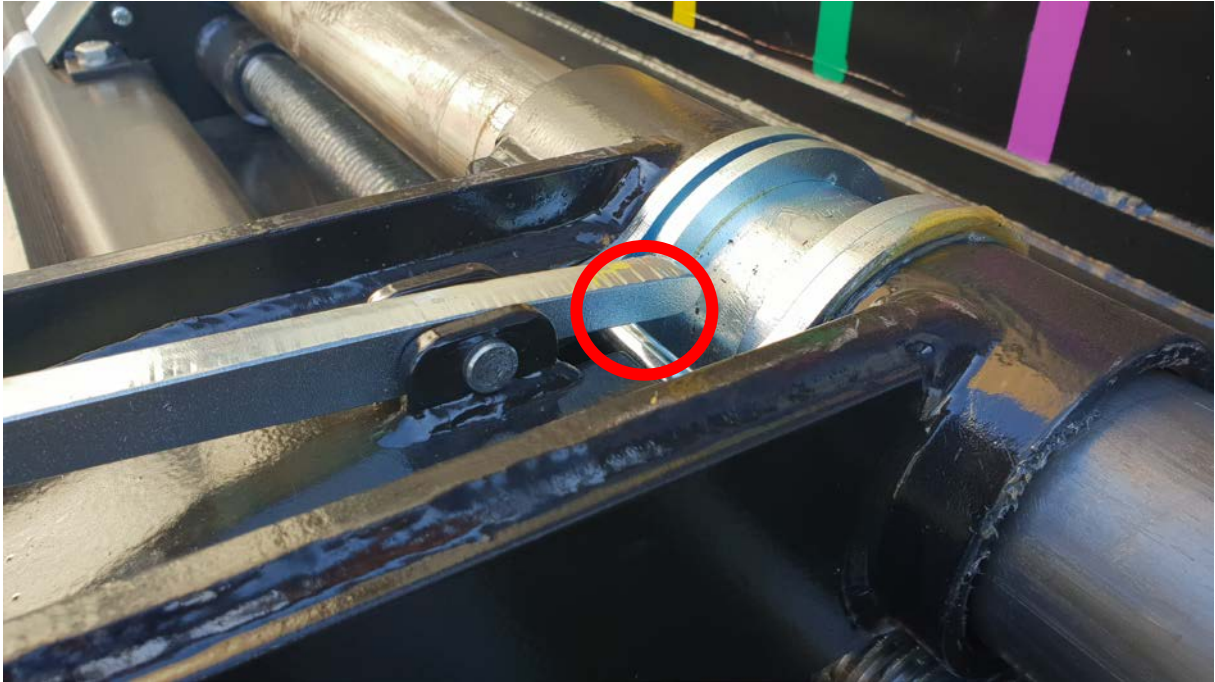
Figure 7 Lever not in “locked” position, no contact with levers
