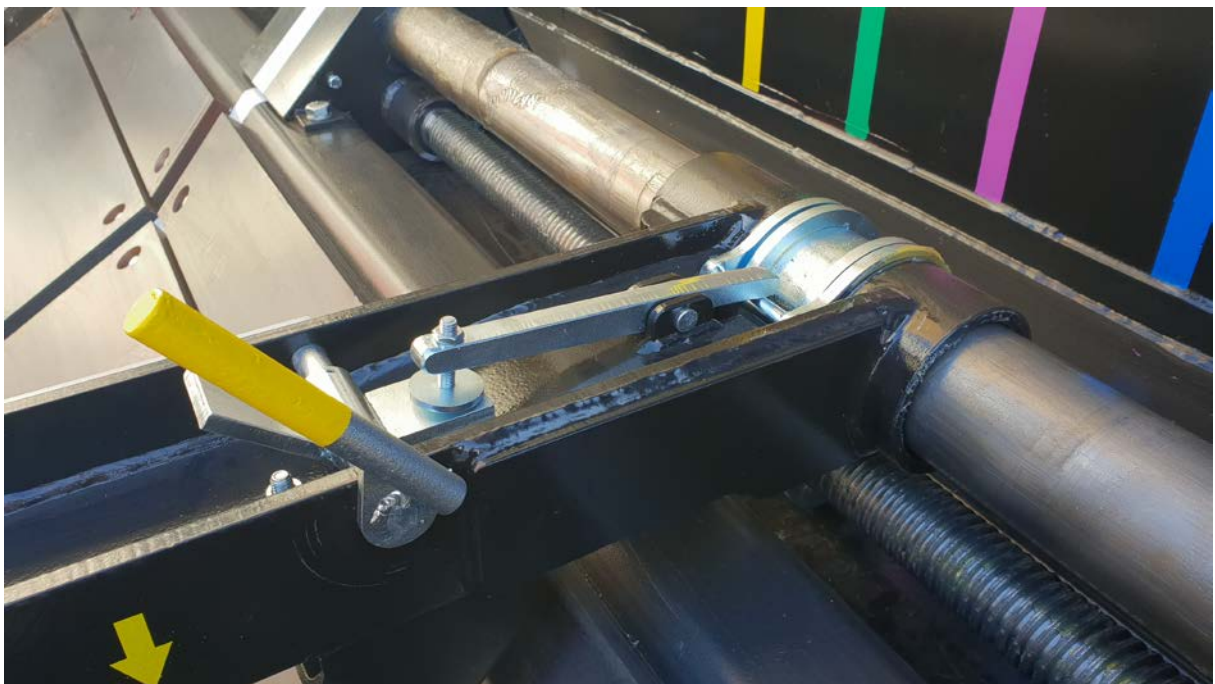
Figure 8 “Locked” position of lever, thread connection screw/nut, contact with levers
