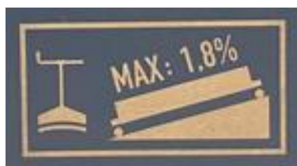
Fig. 5.8: Slope of the parking brake for a T3000e wagon.
