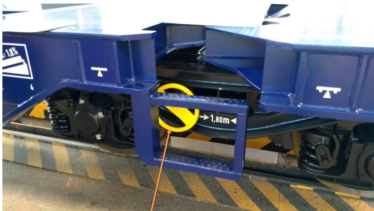
Fig. 5.7: Centre bogie with parking brake wheel
