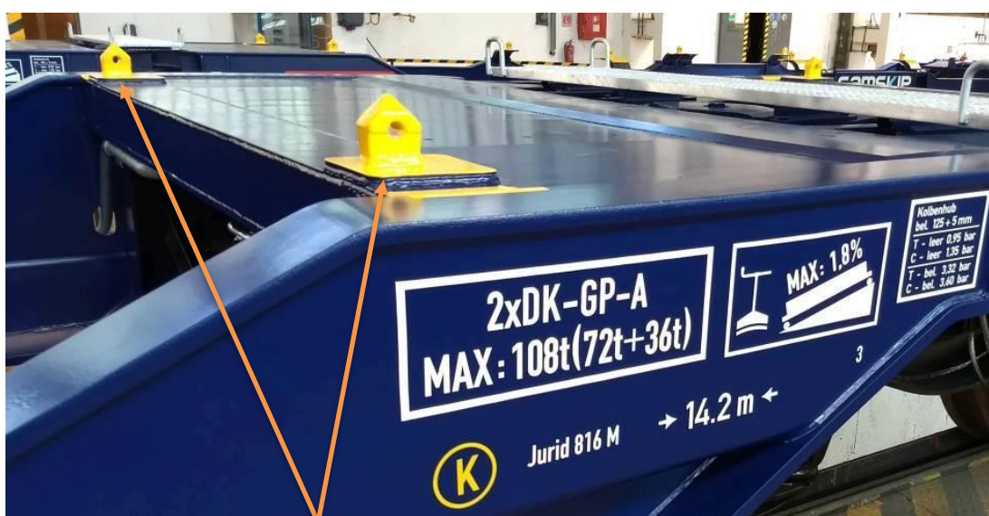
Fig. 6.2: Fixed container jigger pins on the cross member of the central bogie
