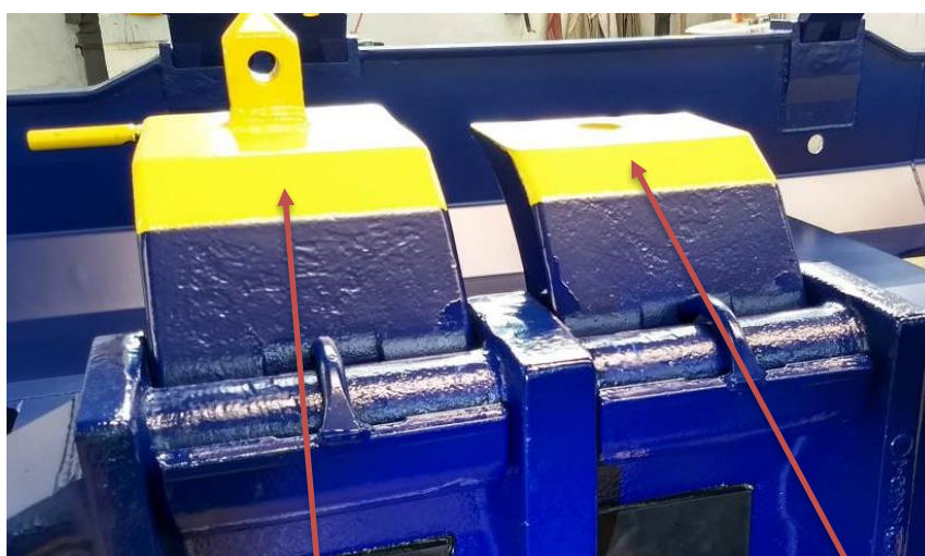
Fig. 6.5: Container jigger pin and foldable swap body support in working position
