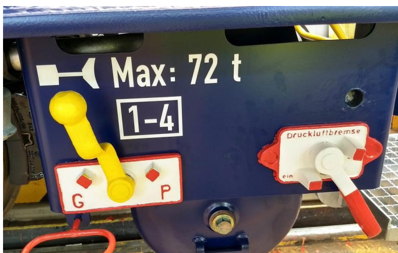
Fig. 5.10: Changeover lever G-P and changeover lever on-off
