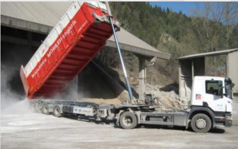
30 ft Multitainer with bulk materials
