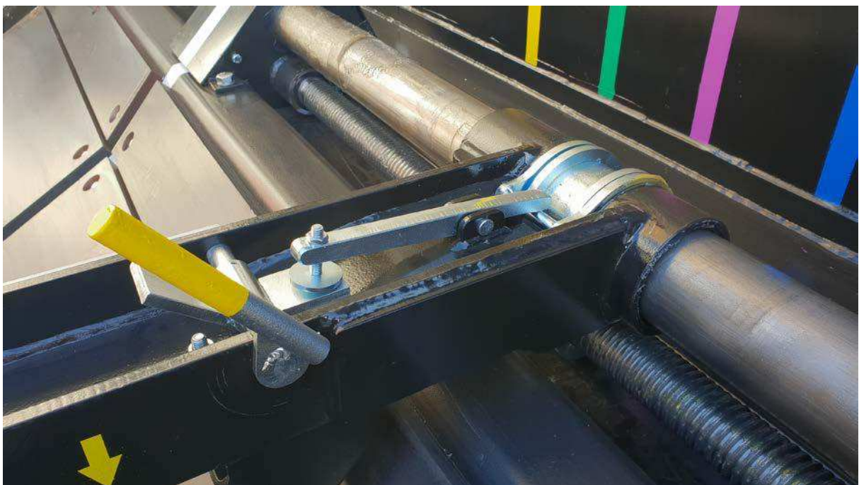
Figure 10 “Locked” position of lever, thread connection screw/nut, contact with levers
