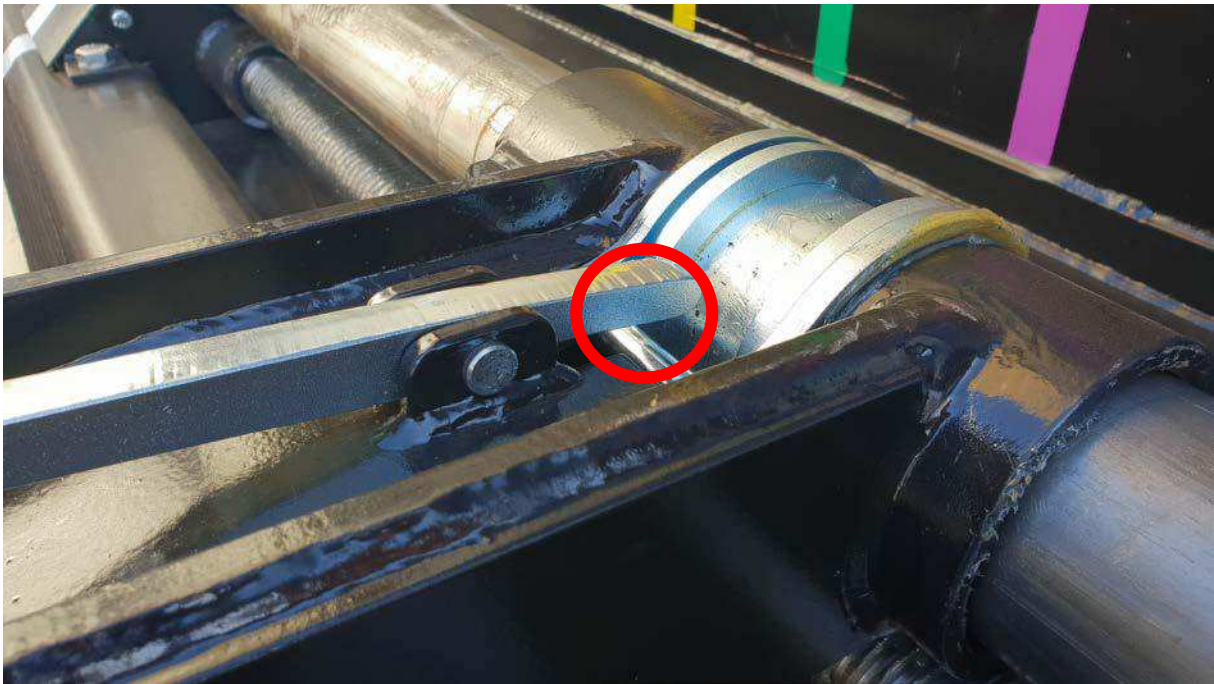
Figure 9 Lever not in “locked” position, no contact with levers
