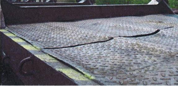
A close-up photograph of a railway wagon floor. The floor is made of a dark, perforated metal material, known as Lupenblech (lupine plate), which consists of a grid of small, circular holes. The surface shows some wear and tear, with a prominent crack running across the middle. The edges of the metal are slightly raised, and the overall appearance is that of a heavy-duty, industrial-grade floor designed for foot traffic. |
