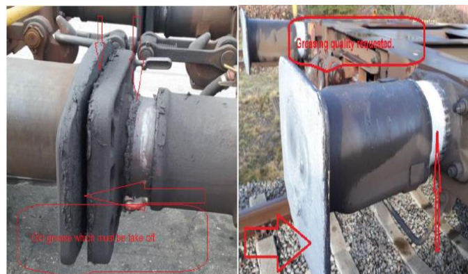
Figure 2: Greasing of the buffers
