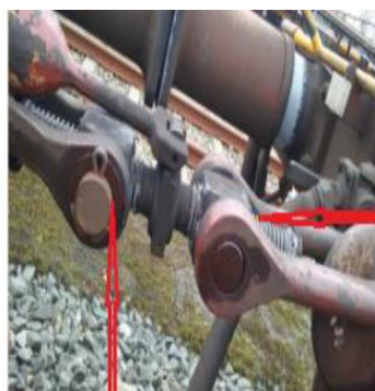
Figure 3: Greasing of the screw coupling
