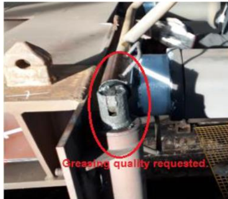
Figure 4: Greasing of the folding handles
