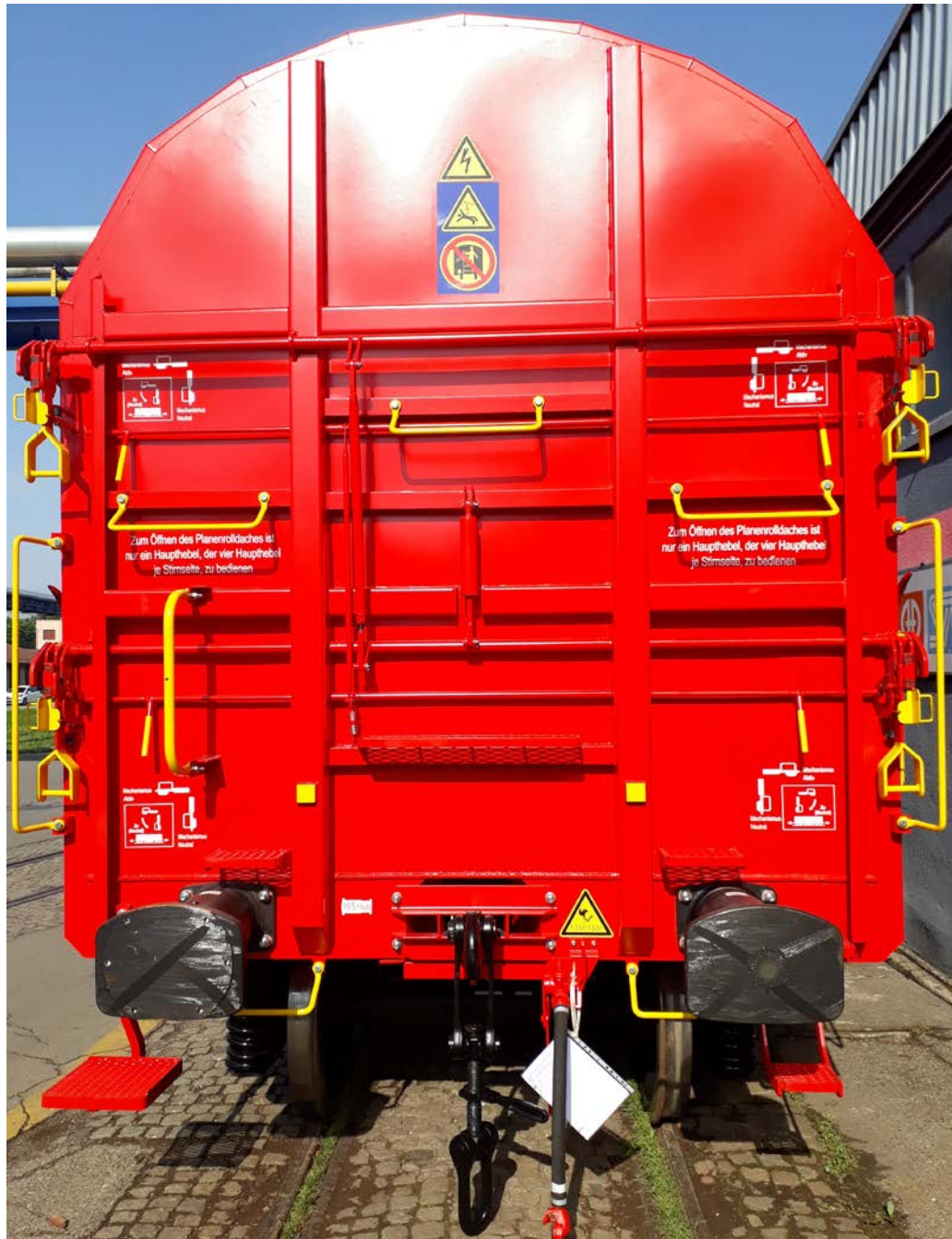
Figure 16 Steps for crossing the wagon
