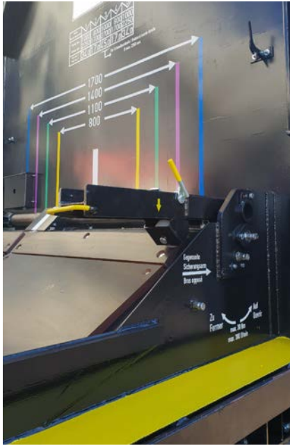
Figure 14 Positioning the arm on the front wall
