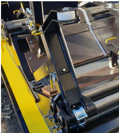
Figure 14 Positioning the arm on the front wall
