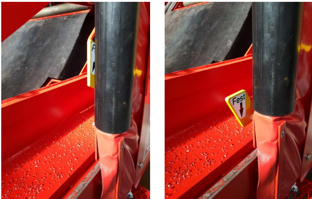
Figure 4 Open and closed position of the tarpaulin brake
