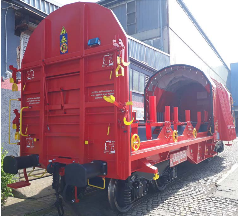
Figure 3 Open position of tarpaulin
