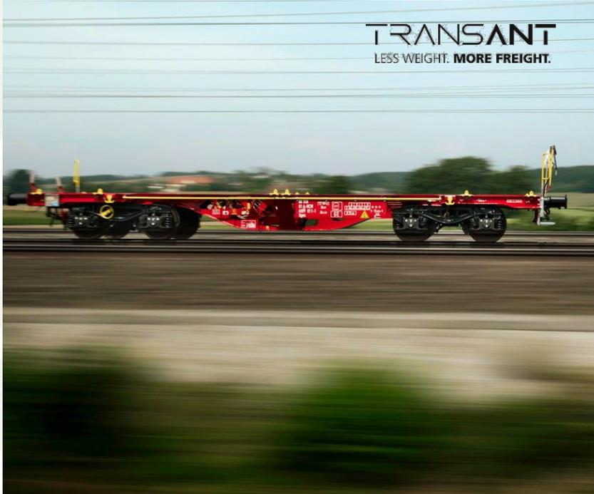
TransANT = a standardised wagon underframe ranging between 33 ft and 70 ft in length with modular, versatile superstructures that can be universally implemented for transporting many different kinds of goods.
